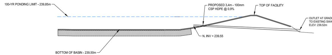
**4** ENHANCED GRASSED SWALE OUTLET CROSS-SECTION DETAIL
