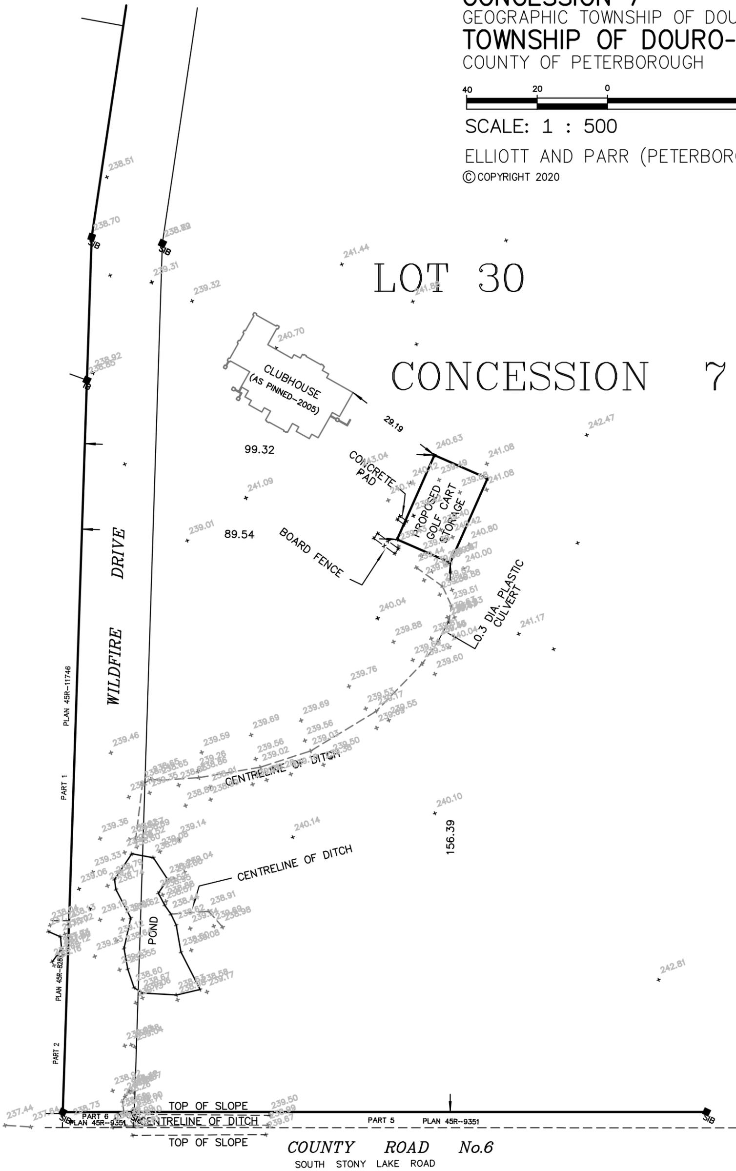
**METRIC** DISTANCES AND/OR COORDINATES SHOWN ON THIS PLAN ARE IN METRES AND CAN BE CONVERTED TO FEET BY DIVIDING BY 0.3048.
