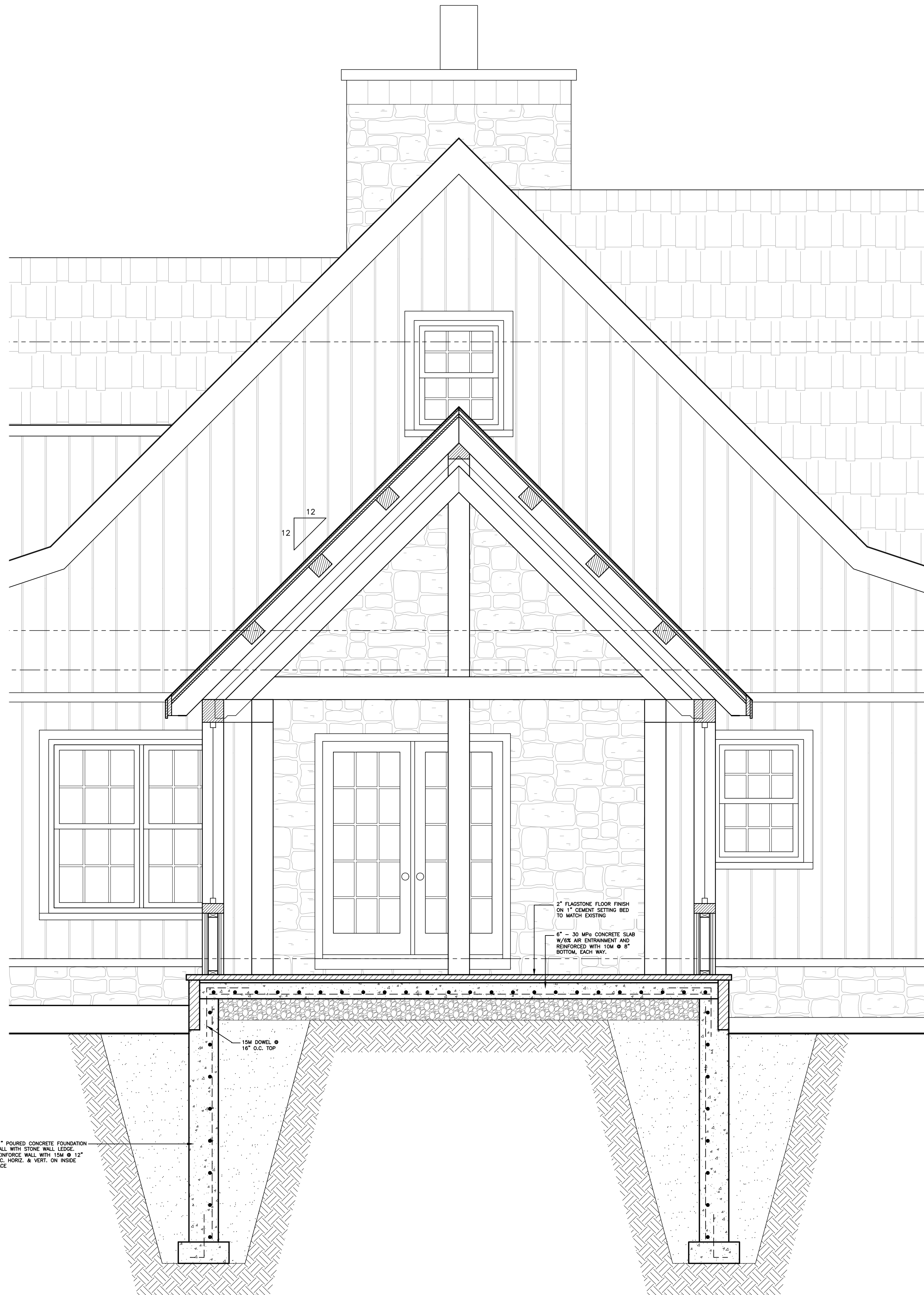
1 SCREEN ROOM SECTION 1 A3 1/2" = 1'-0"
